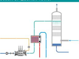
In many different industrial application quench towers are used to condition or clean gases. A high filter availability and performance are key to ensure the productivity of the overall plant. The SAB product portfolio covers many innovative and proven filter solutions which reliably remove solids out of the quench water in order to protect heat exchangers or quench internals, for example the demister. Furthermore, the exceptionally low backflush flow minimizes the fluid losses.
