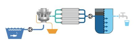
Rising water demands and diminishing water supplies are exacerbating water scarcity in most world regions. Unconventional water resources, such as desalinated water, are expected to play a key role in narrowing the water demand-supply gap. In this process the SAB filter reliably removes solids upstream of the reverse osmosis system which takes out the salt and other minerals.
