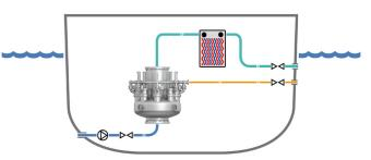
Heat exchangers are frequently used on ships for cooling or heating purposes using sea water. Typical applications are the cooling of engines, special equipment, or heating during the re-gasification of Liquid Natural Gas within the unloading process from an LNG carrier to an FSRU vessel. Here, the SAB filter reliably removes solids upstream of the heat exchangers.
