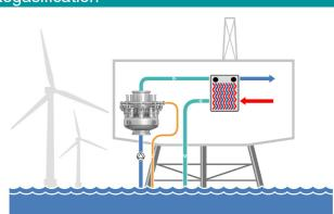
Offshore applications like oil/gas rigs or power converter platforms usually require cooling, process or drinking water. With our comprehensive range of products, SAB delivers customized and optimized filter solutions for numerous different types of applications. One application example is the usage of seawater for cooling purposes. Here, the SAB filters are installed to secure the protection of downstream heat exchangers and to ensure a high efficiency performance of heat exchangers.
